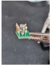
5. Next, bend all resistors outwards a bit so that the transistor can be installed. Make sure that the emitter connection is placed in the hole that is marked with a small "E"
