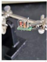
4. Install the 75-ohm resistor. If you are using 2 resistors to make this value, ensure they are soldered end to end (serial connection)
