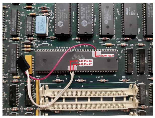
After you solder the wires, you can use the individual connectors or use the included 4 position connector.
