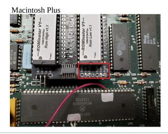
First thing you will need to do is solder the jumper wires to the CPU, there are 4 wires on the 128K and 512K, and 3 wires on the Plus.
