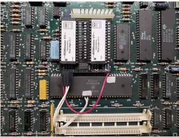
Plug the header wires into the ROMinator V1 board making sure to correct the lines going to the correct labeled pins.
