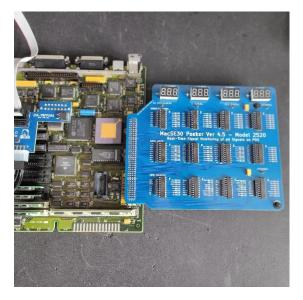
Power up the SE/30 and you should see LEDs flashing and the meters showing voltages, like the image below.
