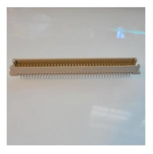
Using the PDS slot of the Macintosh SE/30, insert the connector into the PDS slot of the SE/30. This will leave the pins facing upwards. Place the Peeker board on top and solder the pins to the board. I would recommend just soldering a few then pull it off and finish the rest. This way, you don't over heat the PDS female connector on your SE30. *The reason for installing the PDS connector this way, is to ensure you don't solder it on backwards or on the wrong side.*
