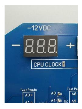
g. Solder the 3 legs then place solder on the additional holes. These pins may not protrude the back of the board, but just place solder to fill each hole as it this help hold the meter to the board.
