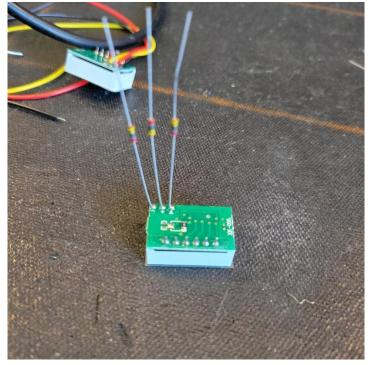
d. Solder in place the 3 resistors so that the leg just barely extends pass the board.
